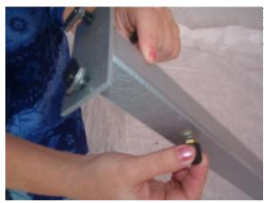
Install a bushing assembly in to each of the four threaded holes on the X-frame. Tighten it just finger tight.
