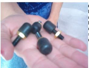
Gather four bushing assemblies. Each one should have a screw, a nut and a rubber cap. We recommend that the rubber cap be installed, however feel free to experiment. Alternately the metal screw could make direct contact with the shelf. In addition, any aftermarket coupling device may be used so long as it has 1/4-20 threads.
