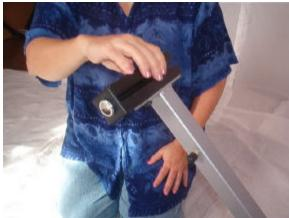
Slide a column onto the end of the X-frame. It does not matter which direction the T-nut nut faces. It is however important that the top of the column points in the same direction as the X-frame bushings. Do not tighten down the fasteners at this time. Finger tight, that's all!
