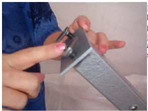
Insert a button-head bolt into one of the **endplate** holes on the X-frame such that the threads are pointing outward. Intall a T-slot nut onto the bolt just enough to hold in place. Do not tighten it down at this time. The side of the T-nut with the bump should be facing outer direction.
