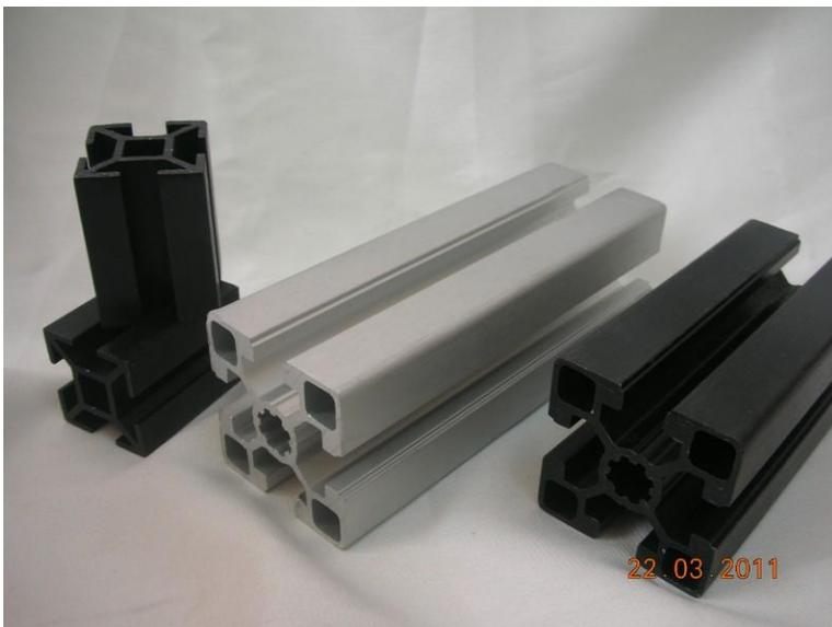
These are Extruded aluminum cross-beams, machined ends with pre-installed connector assemblies. A universal T-slot runs along the top edge, making it easy to install after-market coupling and wire-management devices.
