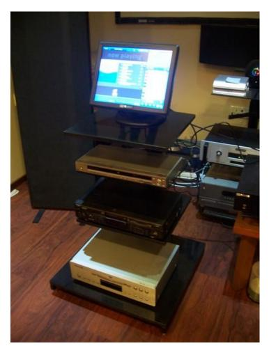
This rack was primarily designed for stealth and aesthetics & looks fantastic when loaded with equipment. A clear favorite with the women of the house is rack uses a combination of two principles; the 3 point cantilever (remember your physics) and a 3 point support. The idea here was a minimalistic look (i.e. once the equipment is loaded - you can't see the rack) It's as if the equipment is suspended with no visible columns as in conventional racks
