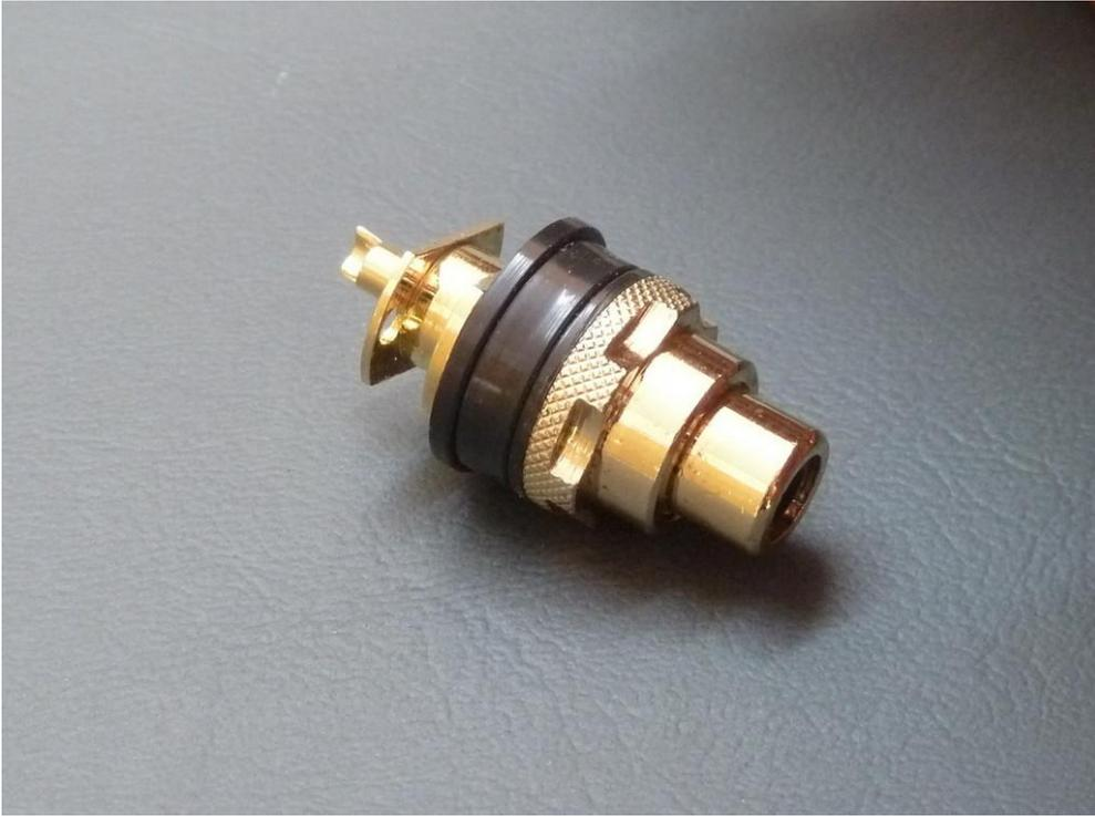
A Diyer's delight. This top end RCA plug features a OFC construction in this dual prism spring loaded contact. The Socket tightens from the outside using the included mounting nut. It comes with insulated key hole slotted washer that prevents rotation of the plug. Design is based on the WBT 0201 rca socket
