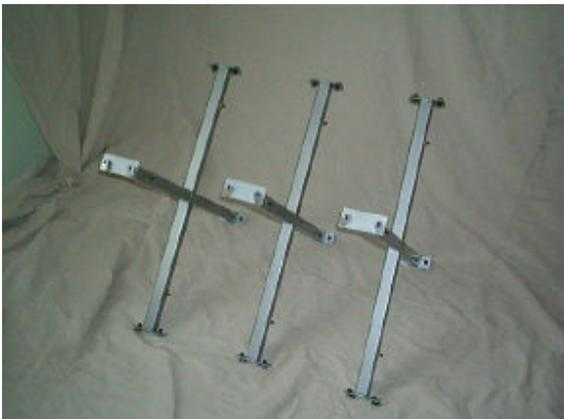
**Lay the x-frames sideways on the floor as shown. Space them roughly the desired distance apart. You will set the actual spacing in a later step. Make sure that all frames have the bushings facing the same direction.**
