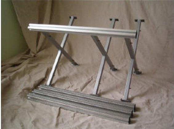
**Slide one of the columns onto the x-frames. Make sure that the column end-cap points in the same direction as the x-frame bushings. Do not tighten any of the hardware until all columns are installed.**
