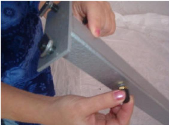
**Install four bushings onto each of the x-frames.**
