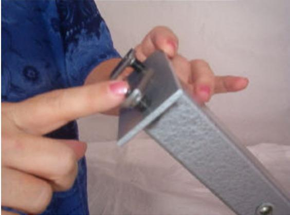
**Insert a button-head screw into one of the holes on the x-frame. Loosly thread a T-slot nut onto the screw just enough to keep it in place. Repeat until all eight screws are installed in each of the frames.**
