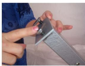
Insert a button-head screw into one of the holes on the x-frame. Loosly thread a T-slot nut onto the screw just enough to keep it in place. Repeat until all eight screws are installed in each of the frames.
