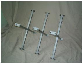
Lay the x-frames sideways on the floor as shown. Space them roughly the disired distance apart. You will set the actual spacing in a later step. Make sure that all frames have the bushings facing the same direction.
