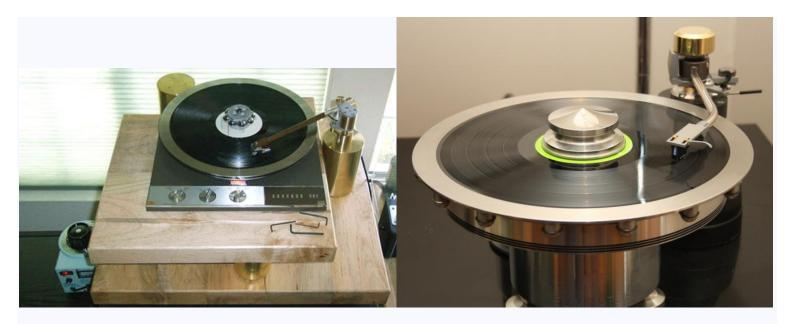
The RSR is intended to reduce resonance in the vinyl surface and to couple the record firmly to the platter. This is achieved by the use of a clamp in the centre of the record as well as the RSR at the periphery of the record. Use of the RSR without a suitable clamp will result in very noisy reproduction along with a strange stereo image presentation
