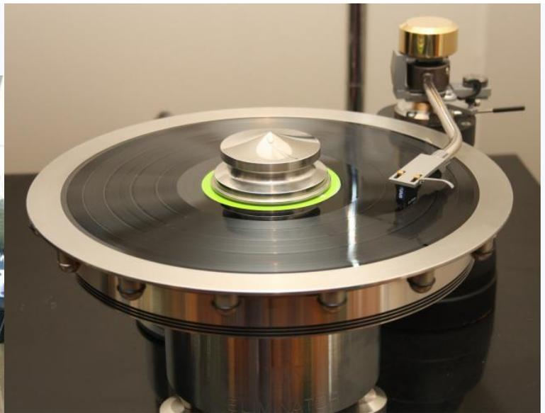
The RSR is intended to reduce resonance in the vinyl surface and to couple the record firmly to the platter. This is achieved by the use of a clamp in the centre of the record as well as the RSR at the periphery of the record. Use of the RSR without a suitable clamp will result in very noisy reproduction along with a strange stereo image presentation
