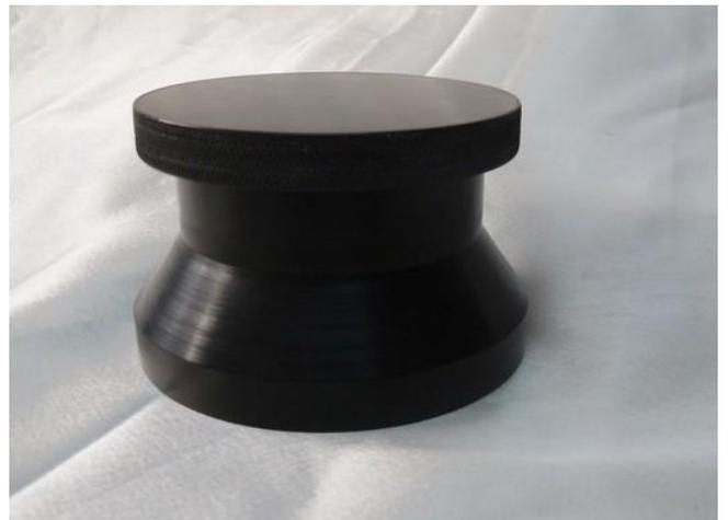
Recommended for Project Debut series, Rega and thorens this weight is an ideal damper for light suspended tables. Diameter is 80mm and height will vary from 1.5- 2 inch depending on contour design. The weight is designed with a low centre of gravity and large flat base. The top end is knurled for grip and the large flat base provides excellent coupling with the record
